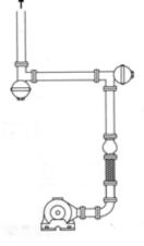
When the fluid flow through the serial corner, the change of flow speed and direction and friction effect will cause unstable pressure wave, which will lead to vibration and noise. To set up arrestor and silent check valve can eliminate the pressure wave.
